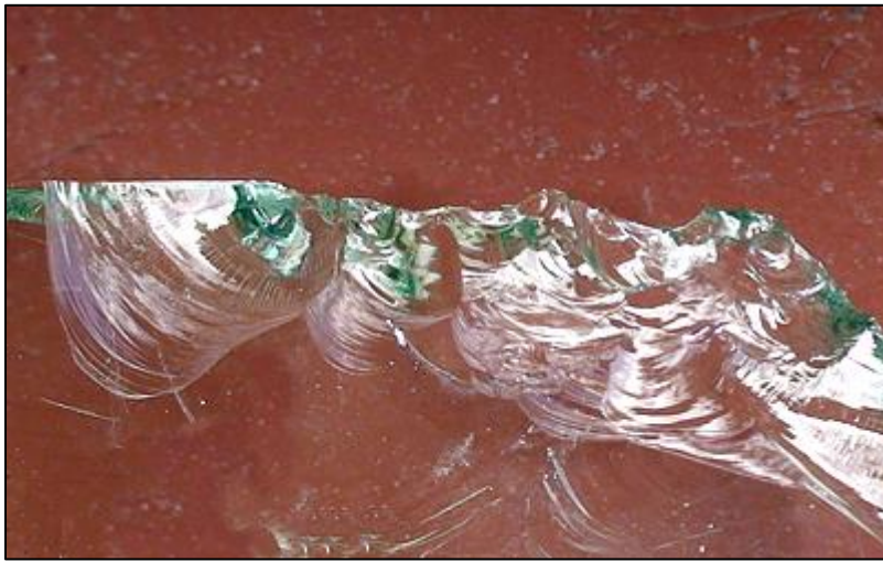
Man-made glass also exhibits conchoidal fracture when struck as can be seen on the edge of this pane of glass.
