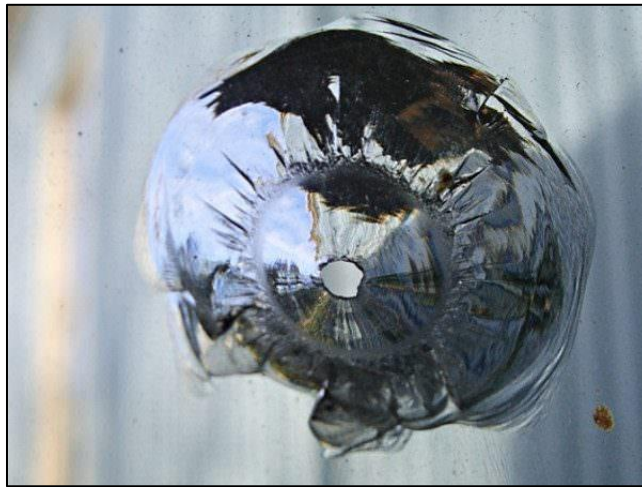
Pane of glass struck by a rock leaving a perfect Hertzian Cone.
